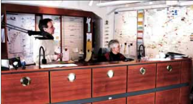
Figure 157. The VTS Stockholm in February 2003. Plotting of ships coming into and leaving Stockholm was at that time still made by boat-shapes magnets moved over a metallic chart on the wall. A simple and functional devise.
