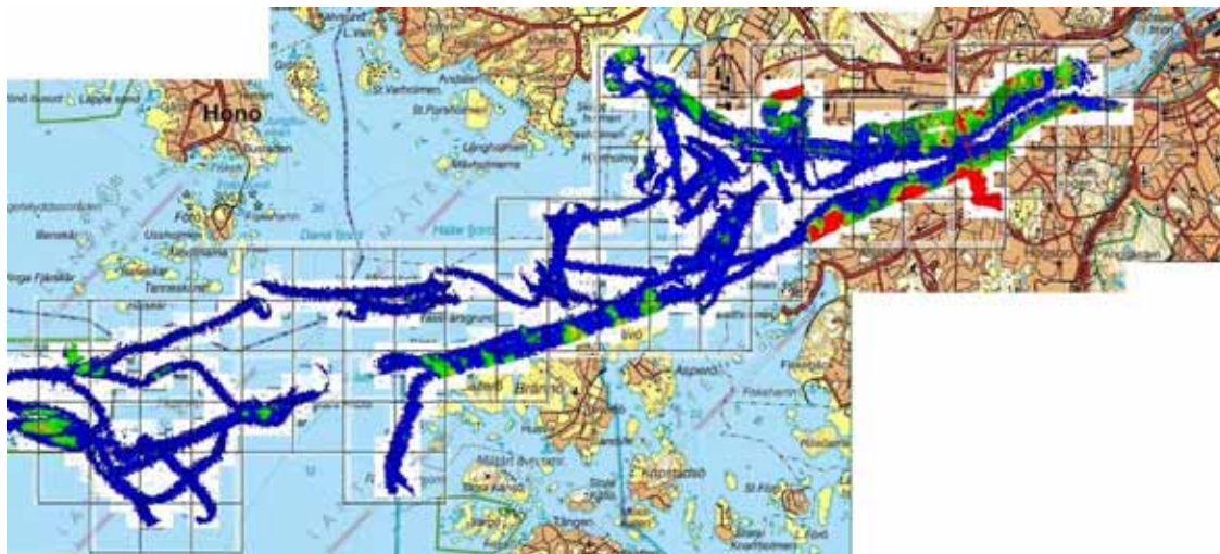
Figure 140. Gothenburg and the approach through the archipelago. Overlaid is the LIDAR data scanned by TopEye in November 2004. The data is pseudo colour based on height. Dark is the 0 m level and lighter is increasing height. No scanning was needed over open water areas; that is why there are “holes” in the scan path.
