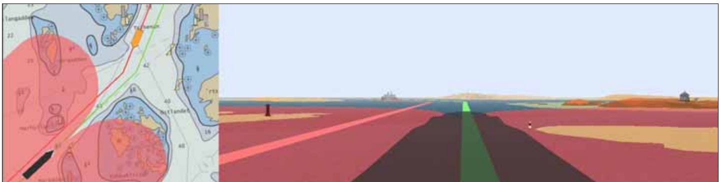
Figure 173. Visualizing the decision space of a ship's maneuverability in a real-time 3-D nautical chart. The red area on both sides of the ship is area out of bounds; the trumpet form in front of the ship predicts the borders of maximum turning angle (Porathe, 2004b).
