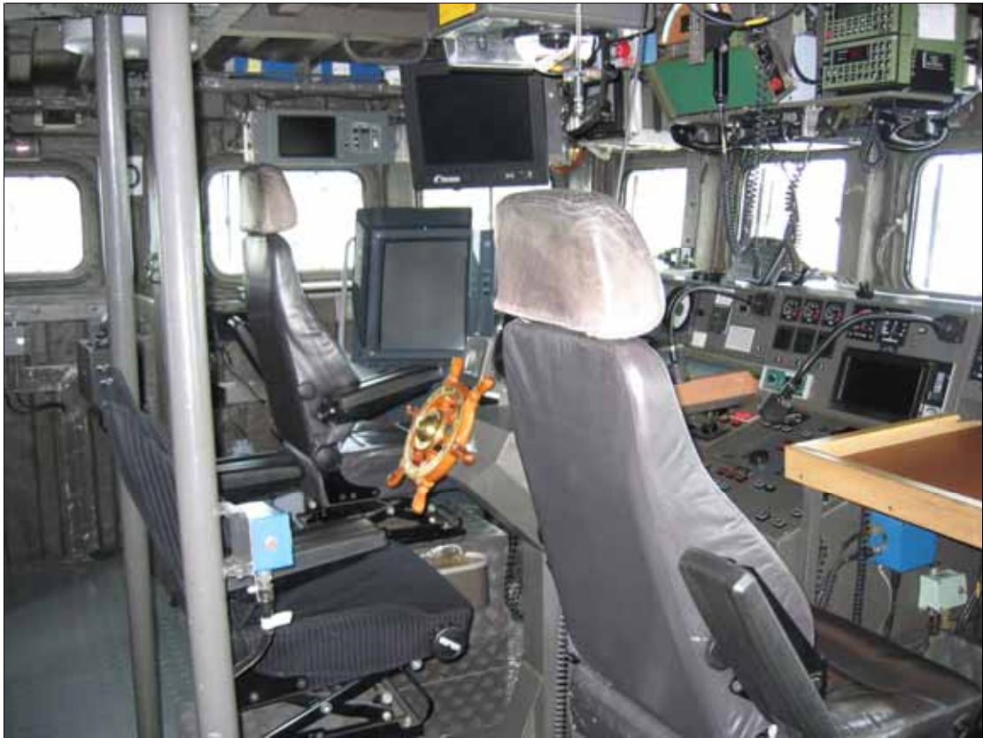
Figure 153. The bridge interior of a navy coast corvette. In the port/left seat sits the conning officer, in the middle the helmsman's and in the starboard/right seat the commanding officer. The third member of the navigation team is seated in the CIC, in the interior of the ship.
