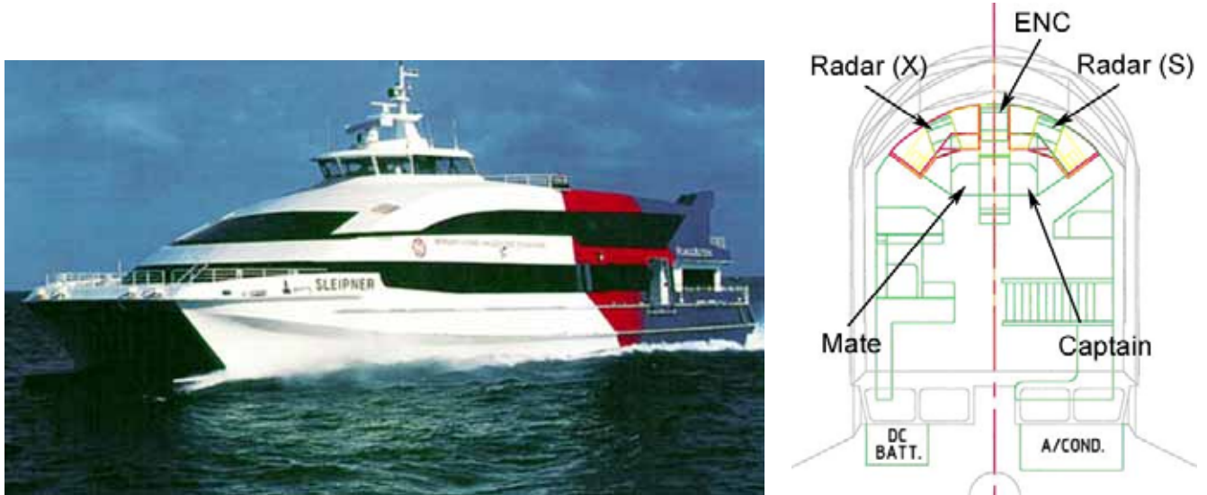
Figure 169. Left, Sleipner Right, the blueprint of the wheel house arrangements. From the report of the accident commission.
