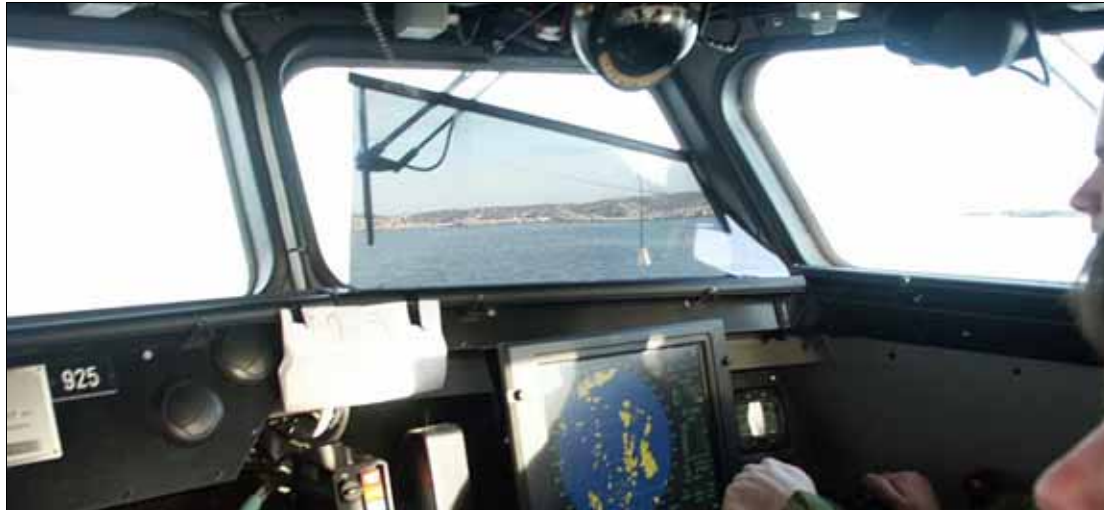
Figure 150. The starboard seat (the driver) of the combat boat. The port, navigator, seat is shown in Chapter 1, Figure 6. In front of the driver a slave screen that can either show the navigators radar or chart screen.
