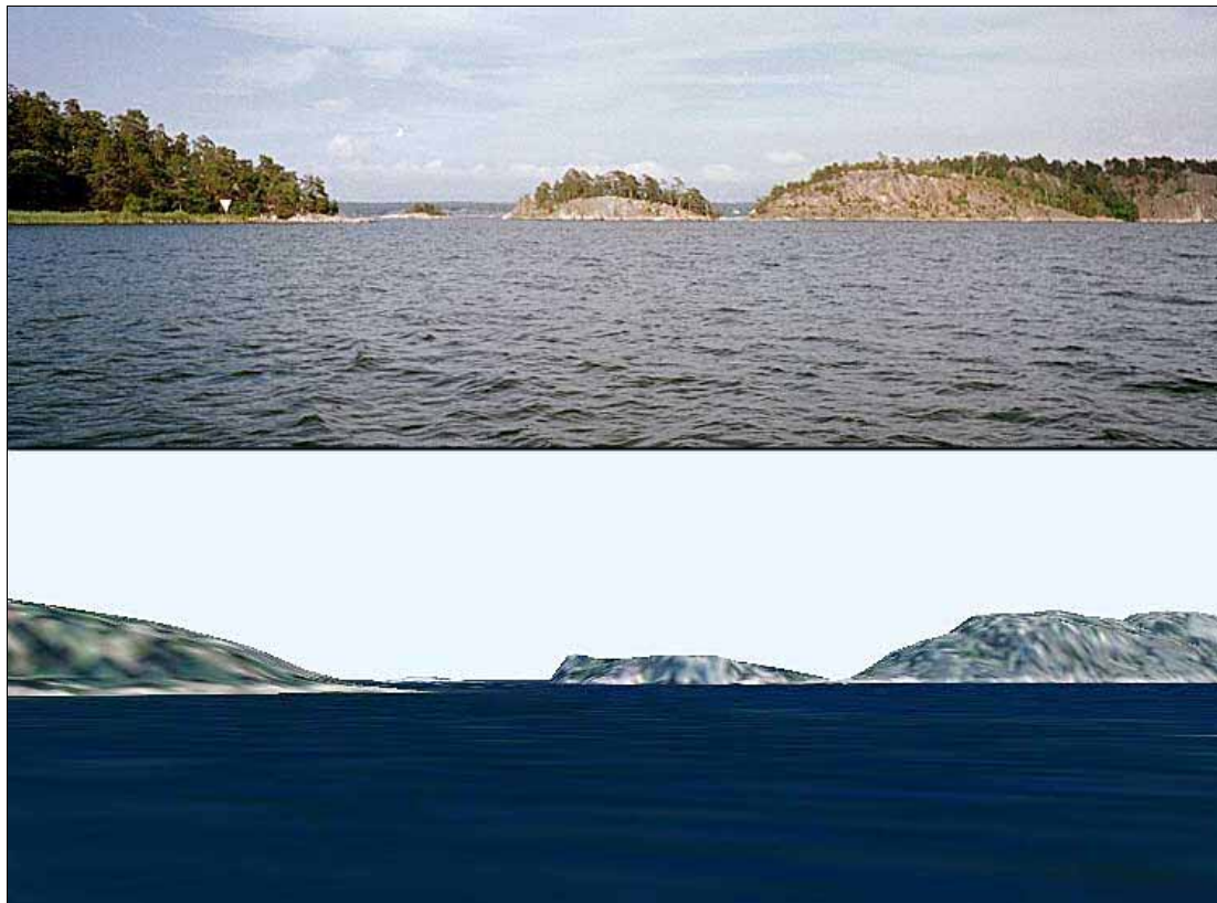
Figure 97. Illustration of the problem of recognizing islands when the model is based on bare earth elevations. When trees are removed the silhouette changes. Bottom, a screen dump from Prototype 5; top, a photo from the same view on location in the Ägnö archipelago.
