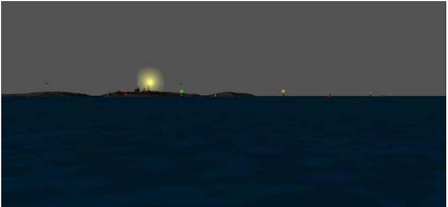
Figure 121. Prototype 6 in night-mode. Lighthouses and light characters are shown, and by dimming the daylight to dusk conditions the terrain will still remain visible. This mode could be useful for training and comparison with the physical world.
