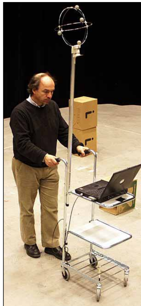
Figure 55. The cart with the “antenna” of four reflective pebbles and the centre of the local coordinate system visualized by the pen at the bottom of the cart. Photo by Emilie Porathe.
