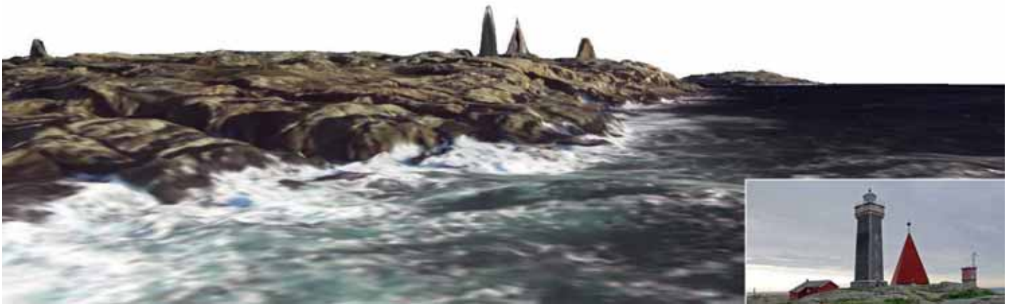
Figure 92. A raw digital terrain model made from LIDAR data, down-sampled to 2 meter resolution and draped with orthophoto with a resolution of 25 cm per pixel. Note the somewhat “melted” look of the lighthouse, beacon and watch-tower of Vinga. Here the sea surface is not yet removed and due to heavy swells the sea surface gave good reflection for the laser pulses. The inserted photo shows the real silhouette of the beacons.
