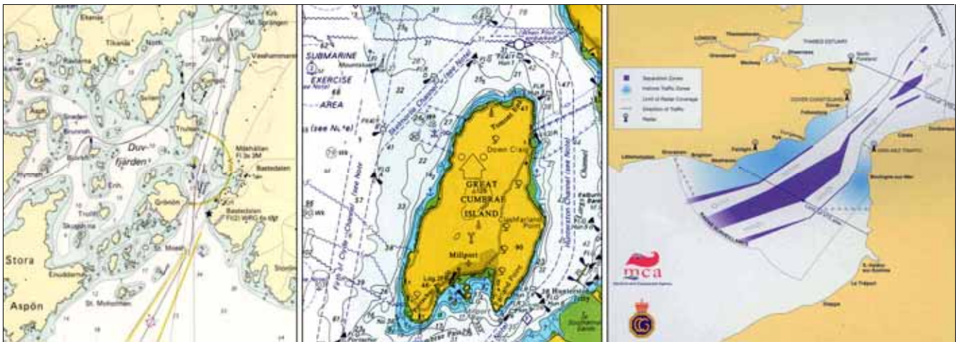
Figure 17. Examples of “roads of the sea.” From left to right: single-line fairways in a Swedish chart, dredged, double-lined channels in an Irish chart and the British Coast Guard’s overview of the traffic separation scheme in the English Channel.
