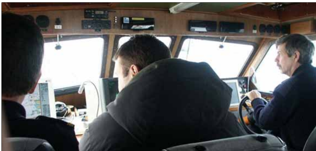
Figure 149. The interior of the police patrol boat. The driver in the starboard seat. In front of him a screen that can either show the radar or the electronic chart. In the middle (in front of the journalist) is the radar screen and to the left, in front of the police assistant, the electronic chart.
