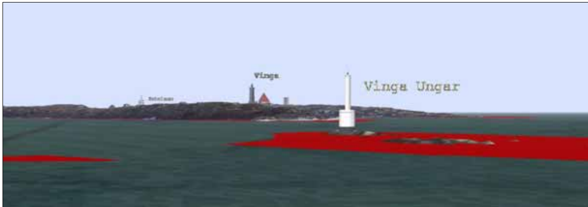
Figure 109. Dynamic No-Go area polygons in the egocentric 3-D mode. Here the polygons are set at 10 meters. Screen dump from Prototype 3 over the Mariehamn entrance in the Åland archipelago.
