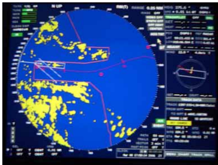
Figure 156. The radar display with additional chart information. Here the ferry is still in port and the traffic limitation borders represent the quays. Photo Margareta Lützhöft.
