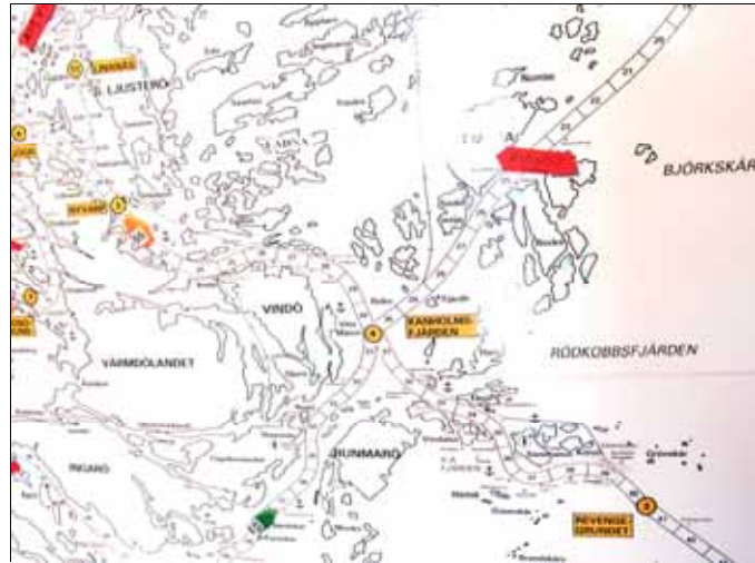
Figure 157. The VTS Stockholm in February 2003. Plotting of ships coming into and leaving Stockholm was at that time still made by boat-shapes magnets moved over a metallic chart on the wall. A simple and functional devise.
