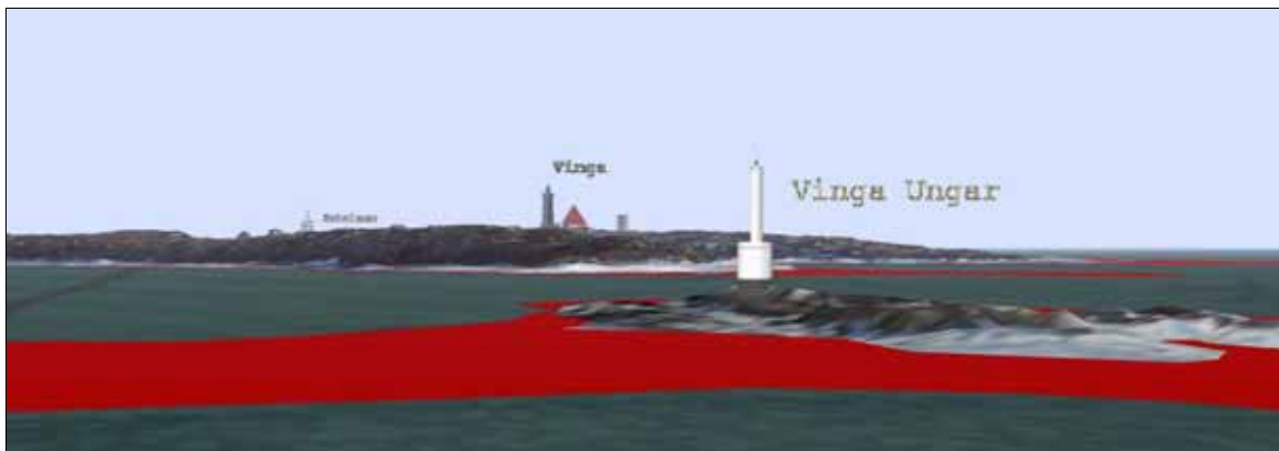
Figure 110. Dynamic No-Go area polygons in Prototype 6, the entrance to Gothenburg. Here Vinga Ungar lighthouse. In the top picture the polygons are set for a draught of 2.5 meters and 1 m high water. In the bottom picture the draught is still 2.5 meters and the water level is 1 meter low water.
