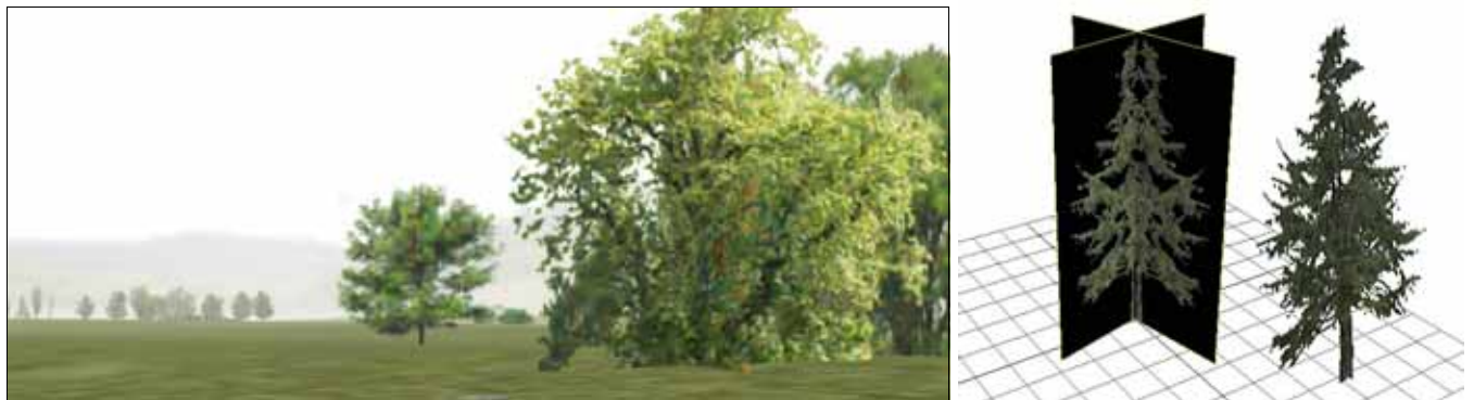
Figure 98. Tree visualization from textured polygons. The representation is appealing but time consuming to make and forests use far too many polygons for real-time systems to cope with.
