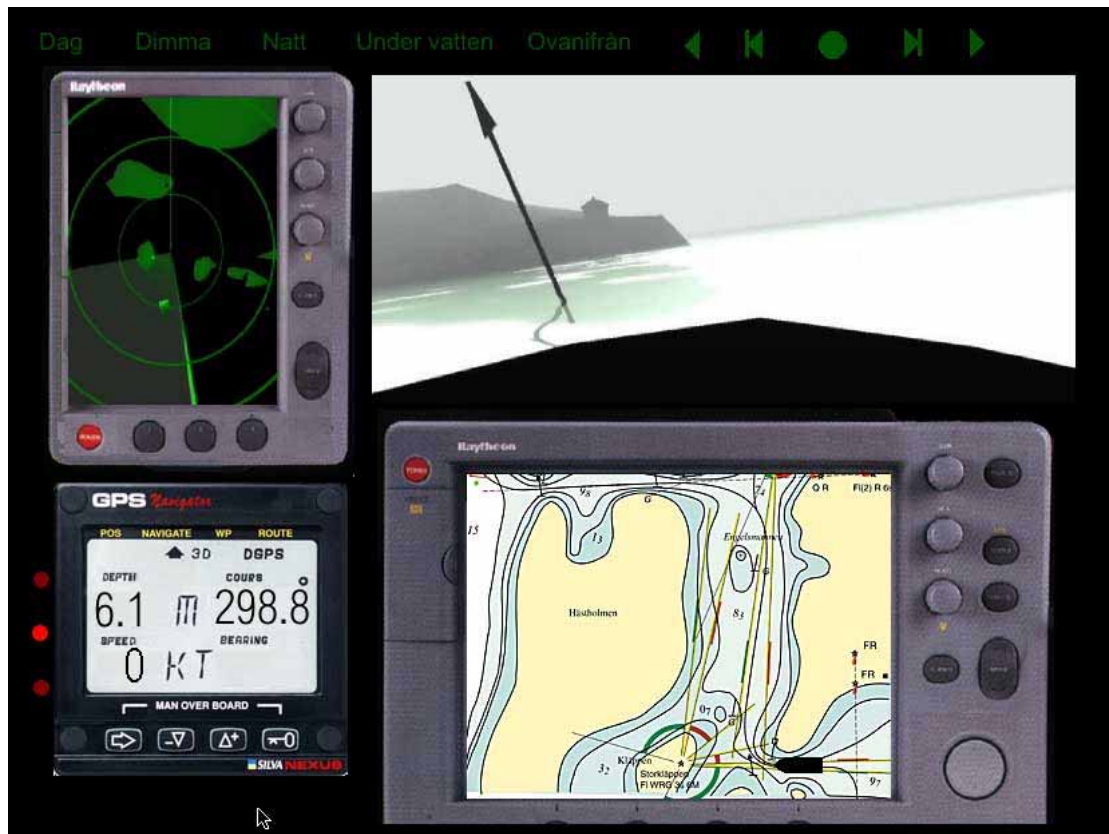
Figure 123. One of the first tests using three inter-connected pre-rendered video films (egocentric view, chart and radar) to visualize the concept.
