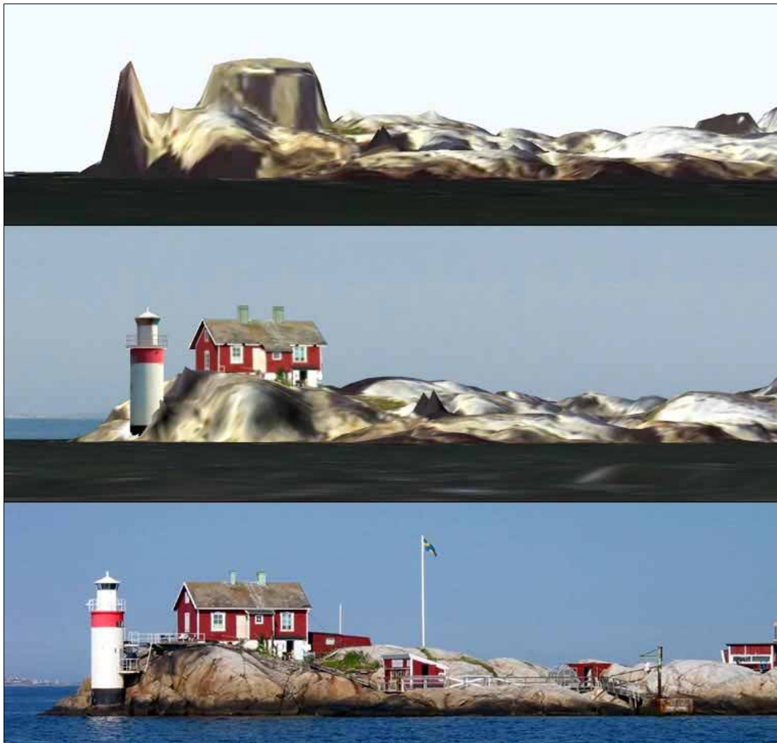
Figure 105. Laser scanned elevation model. Top: the ortho-photo draped polygon model made from raw laser data. Middle, the 3-D chart with hand made buildings. Bottom, a photo from the real world. Gäveskar lighthouse in the Gothenburg archipelago.
